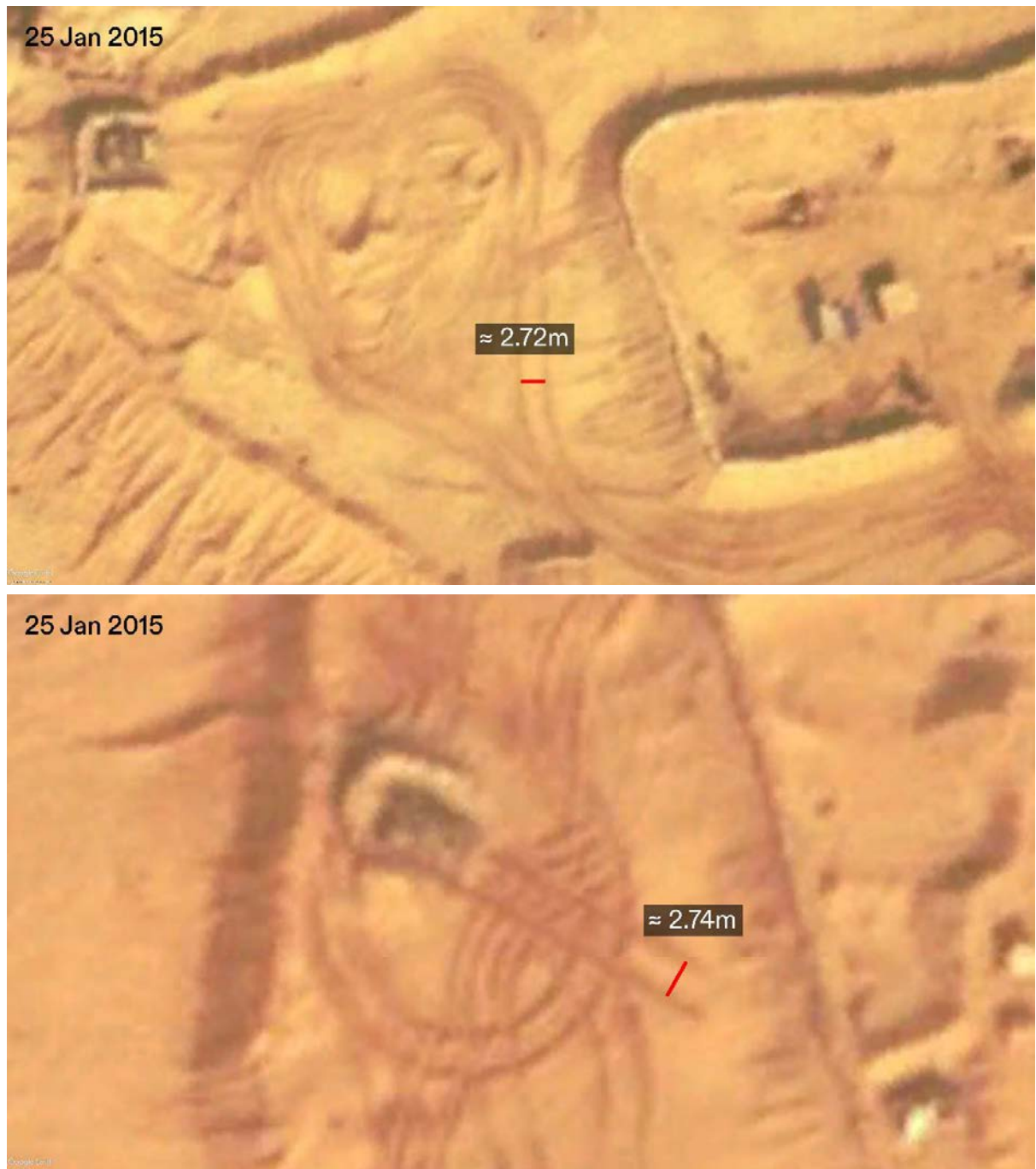
Figure 34: Satellite image from January 25, 2015 of outpost C (top) and outpost F (bottom), showing track marks likely left by large military vehicles. The track spacing is measured from centre to centre.
